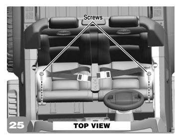
• Insert two screws into the tabs on the front edge of the seat and tighten.
